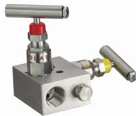
2 VALVE; Horizontal B&B Style; Remote Mount; 316/L; 1/2" NPT (F) x 1/2" NPT (F) with 1/4 NPT (F) Drain & Plug; PTFE Packing
