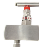
316/L; 1/2" NPT (F) x 1/2" NPT (F) with 1/4" (F) NPT Drain & Plug; PTFE Packing
