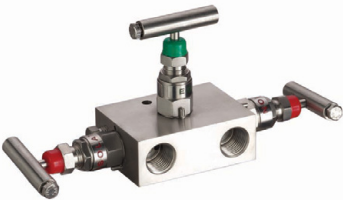
3 VALVE; Horizontal Style; Remote Mount; 316/L; 1/2" NPT (F) x 1/2" NPT (F) x 1/4" NPT Drain/Vent; PTFE Packing
